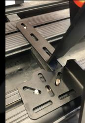
14. Install the washers and Nyloc nuts onto the 3 channel bolts. You may need to insert something into the slot beneath each channel nut to hold them high enough to begin threading the Nyloc nuts on. Align the bracket at 90° to the platform planks, then tighten the Nyloc nuts on the channel bolts sufficiently to ensure that the bracket is securely fastened to the platform and cannot move.
