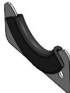
Ladder mounting - bracket shim
